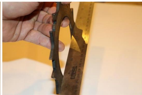
Figure 3 Friction Plate
