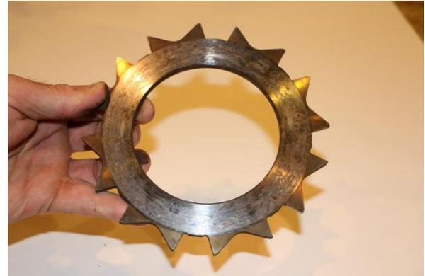
Figure 3.1 Friction Plate Coloring
