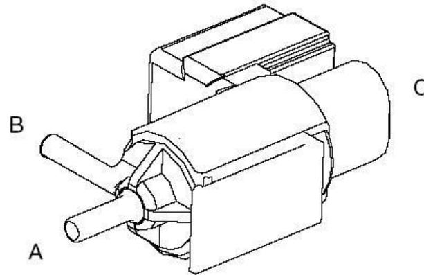
When the valve is OFF, A is closed off the actuator B is vented to atmosphere C
