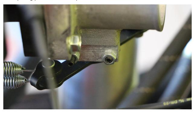
Once the idle is set, ensure that that 100% on the pedal also is rotating no more than a perfect 90 degree. That is the second set screw on the throttle body. Turn that in or out to ensure that this setting is achieved.
